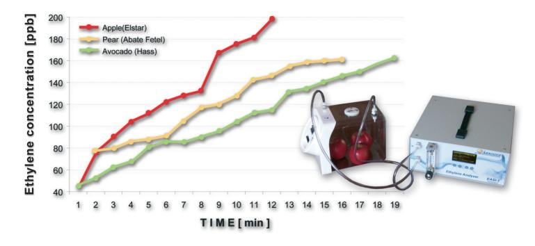
The analyzer provides extremely linear responses at low ethylene concentrations of below 10 ppm. This linearity is critical for simple calibration and measurement over a wide range of concentrations.
