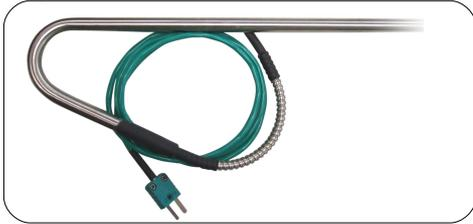
Reinforced cable output with flexible.
